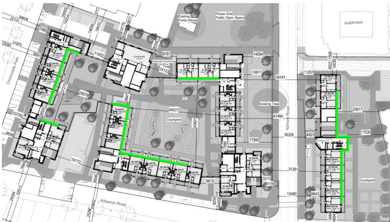
Figure 12: Locations of façades suitable for ventilation via openable windows during the daytime period.
