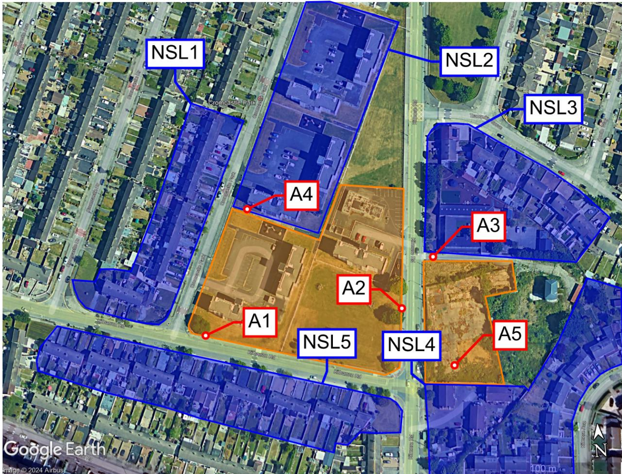
Figure 1: Site Location, noise sensitive locations, measurement locations A1-A5 and the surrounding area.
