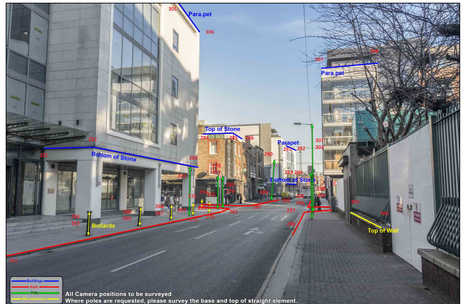
Fig.8: Fixed reference points fully surveyed and numbered.
