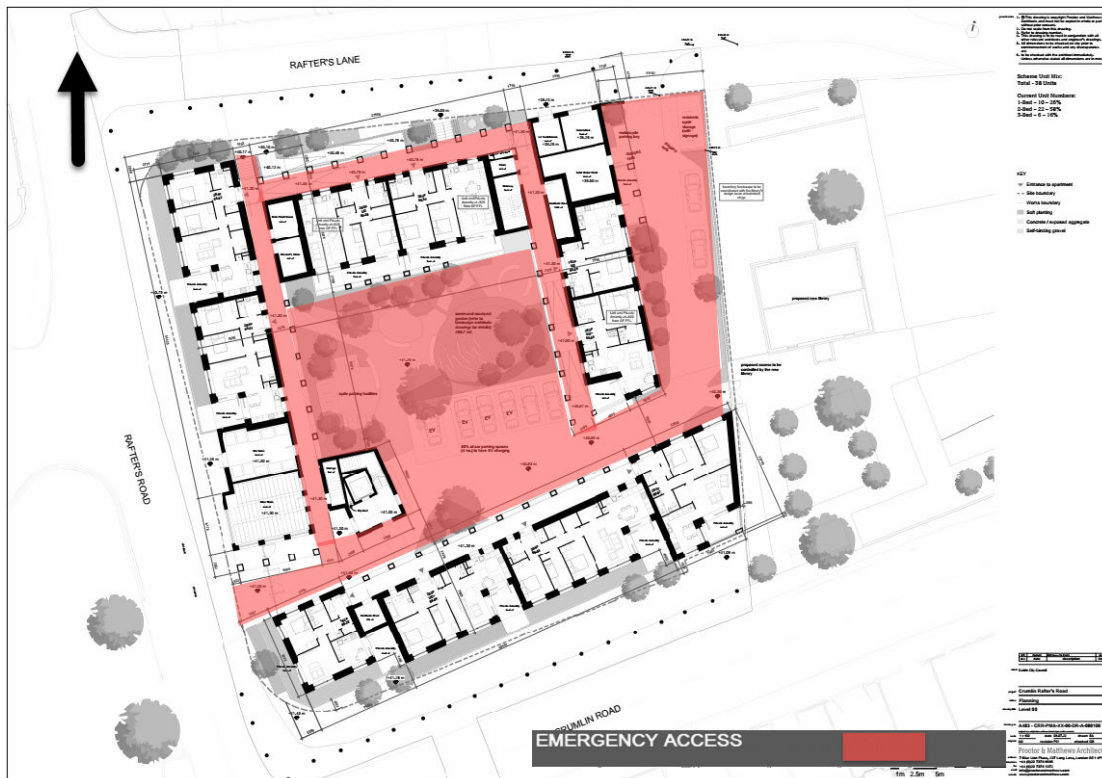
Fig 4. Emergency Access Zone
