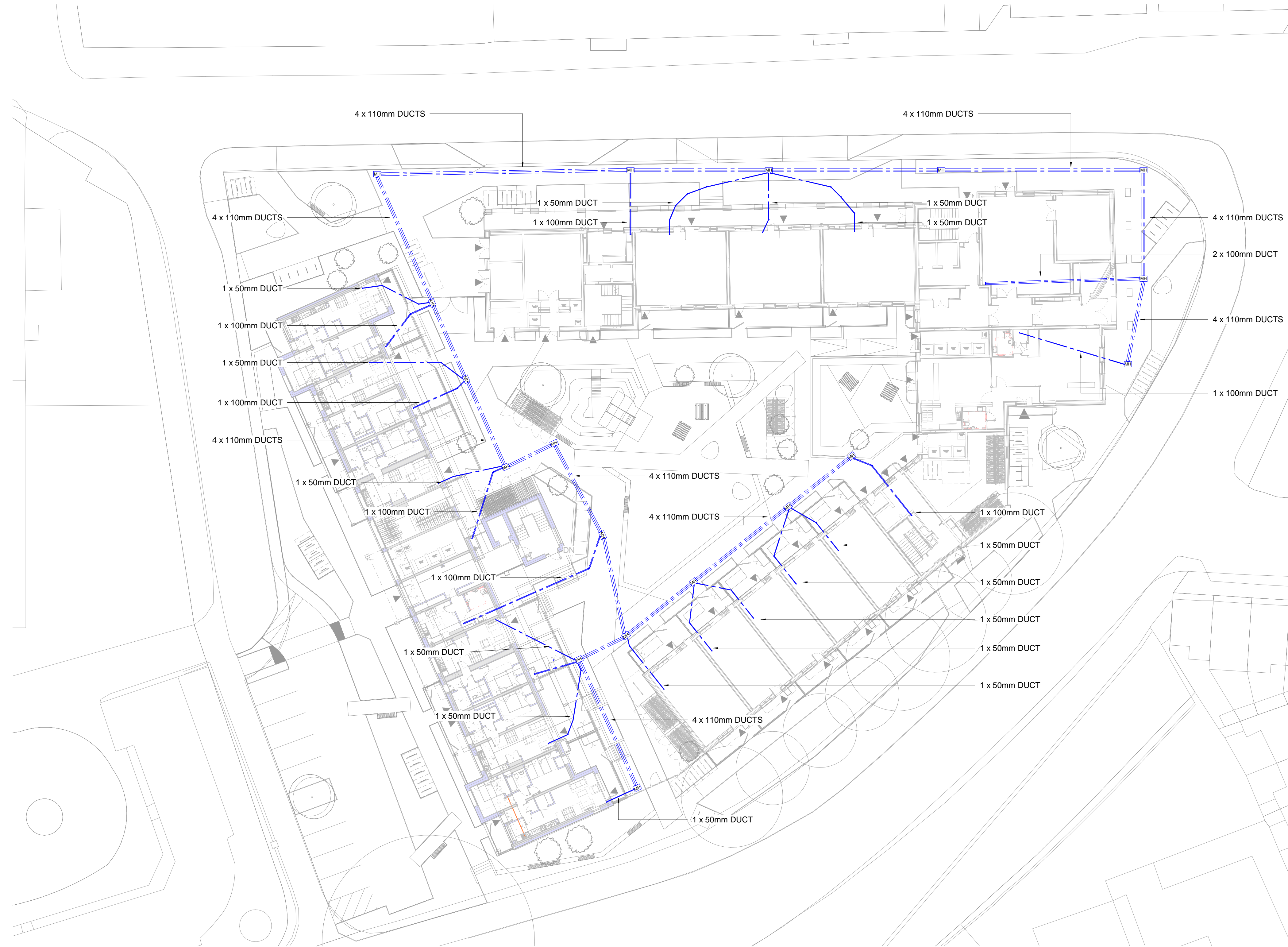
External Site Services Telecoms Cable Containment - A1-00 1 : 250
