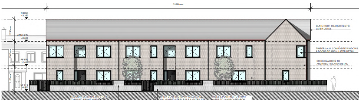
Figure 9 – Housing Block 2 – Elevation CC
